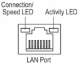
The diagram shows a LAN Port with two LEDs: a Connection/Speed LED and an Activity LED. Below the diagram are two tables explaining their states.
