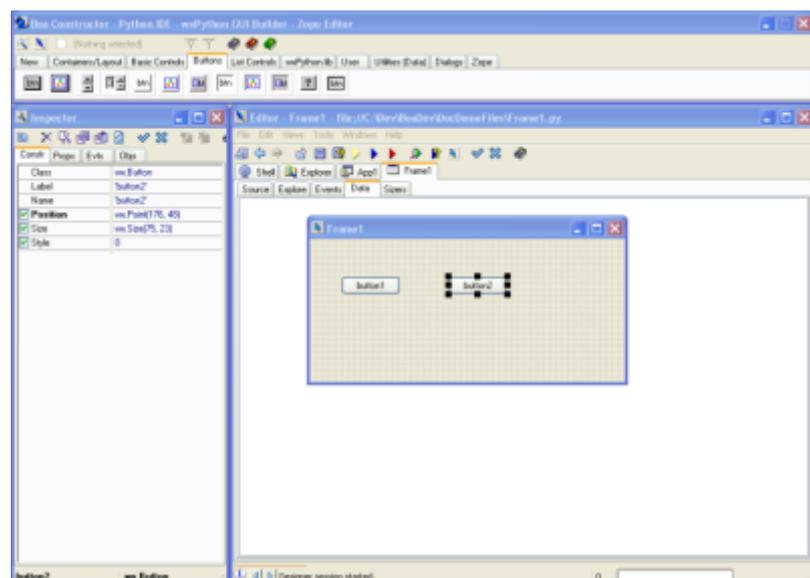
The Frame1 titled window above is the Frame Designer window, a wx.Panel (found on the Containers/Layout palette) has been placed in the wx.Frame and into it two wx.Button controls (found on the Buttons palette) have been placed. The button2 control is currently selected and you can see its
