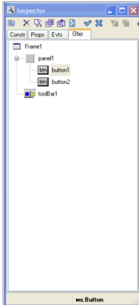
The Objects page allows you to navigate through your components in an alternative format to the Designer pane. This is particularly useful if you have invisible or overlapping components. Also certain components like the wxStatusBar do not process click events (on MSW) so it has to be selected in the Objects page.
