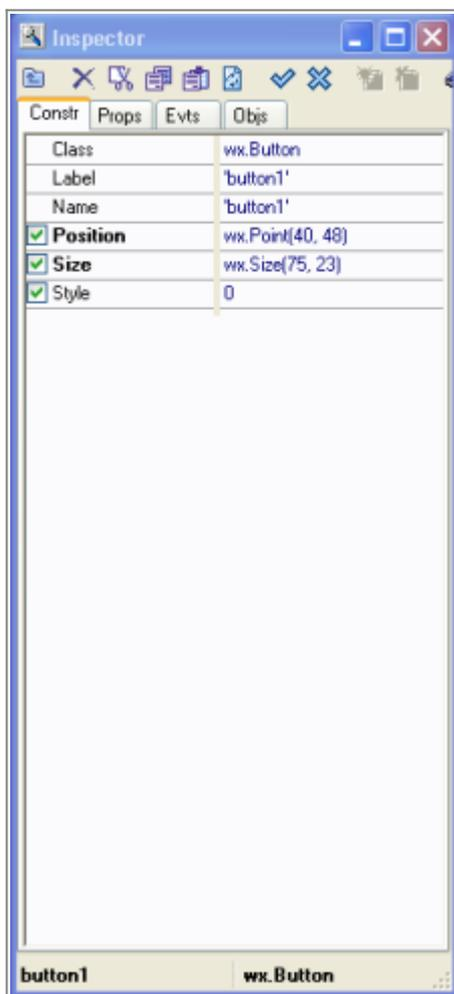
The Constructor page allows you to edit properties which are required at object construction time, e.g. the name and style of the component. Look at the wxPython help for the values passed to the constructor for a control. The styles in the manual are of particular importance. Please note that changes to certain constructor parameters only take effect when the control is created. You should change the "Name" property to something which will make sense to someone else or to you in 3 month time!
